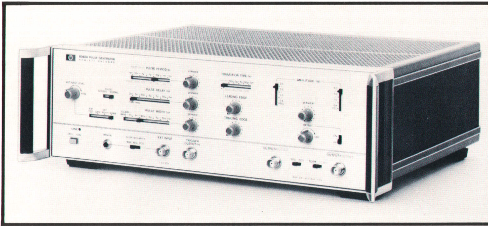
Fig. 1. Model 8082A Pulse Generator gives control of transition times over a range of 1 ns to 5 ms and pulse repetition rates as high as 250 MHz. Two outputs are provided, one the complement of the other. To speed operator familiarization, the slide switches concerned with time functions are arranged horizontally while those concerned with pulse amplitude are arranged vertically.
